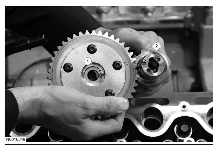
Phaser Pin and Cam Notch
